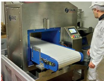
Fig. 1 – Magnetic induction scanner
