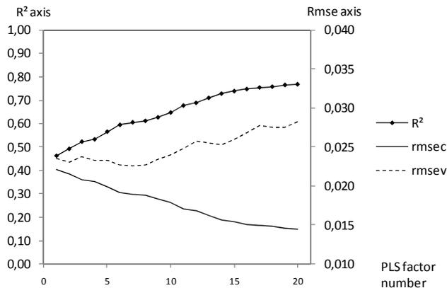
Figure 2: selection curves of the number of PLS factors for the loins cooking yield prediction by visible spectroscopy
