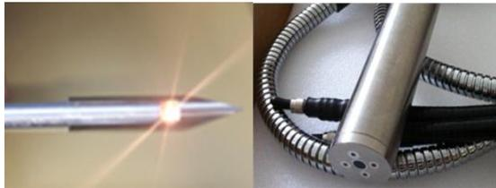
Figure 2. FOP probe (left) and FOS probe (right).
