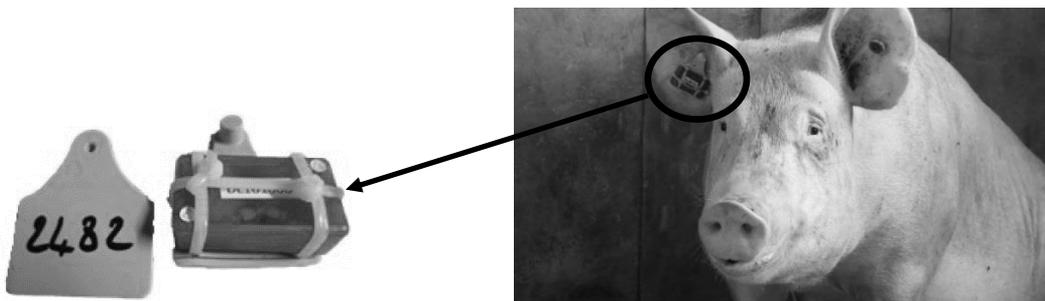
In order to synchronise accelerometer data with video recording, the operator rotated the sensor three times in front of one of the five cameras before attaching it to the animal.
