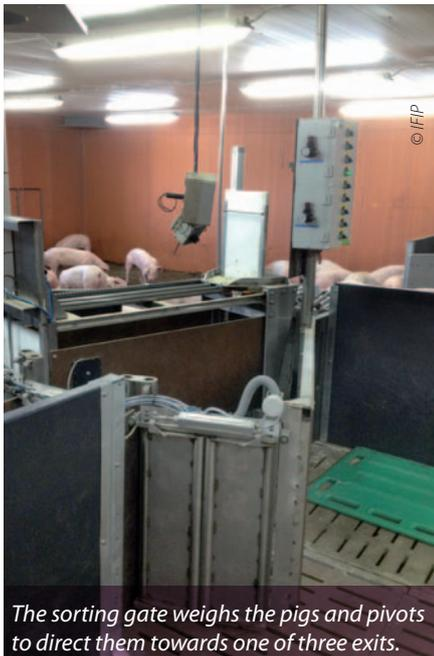
The sorting gate weighs the pigs and pivots to direct them towards one of three exits.
